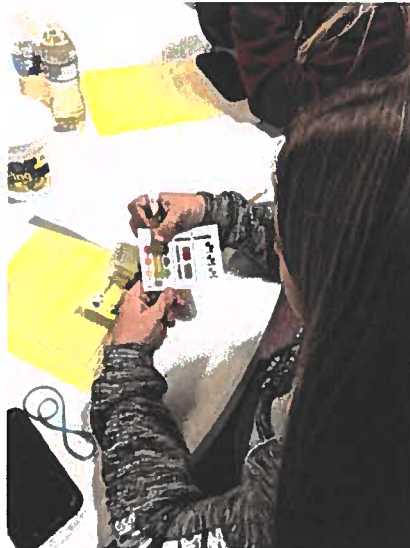
Each youth brought a water sample to test for pH, nitrate, TDS and other parameters.
