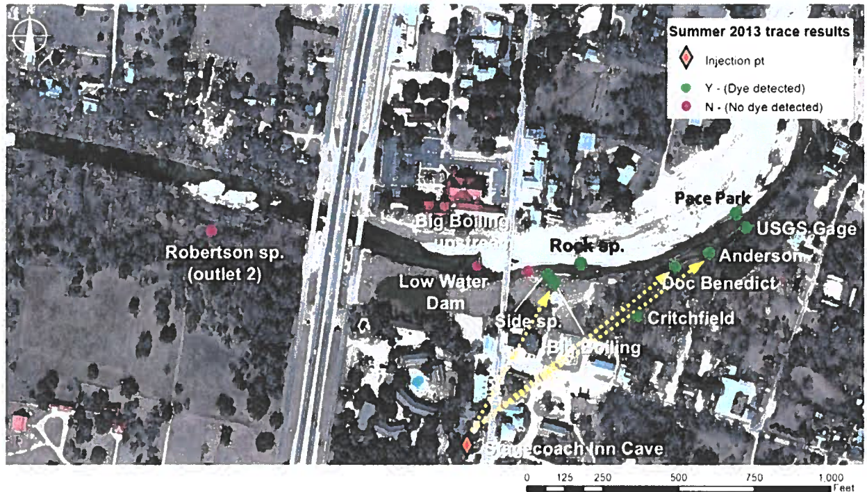
Figure 8: Results of the summer 2013 dye trace test. Purple dots indicate locations of no dye detection. Green dots indicate spring and creek locations where uranine was detected. Arrows represent confirmations of groundwater flow between the injection point at Stagecoach Inn Cave Well and a spring.
