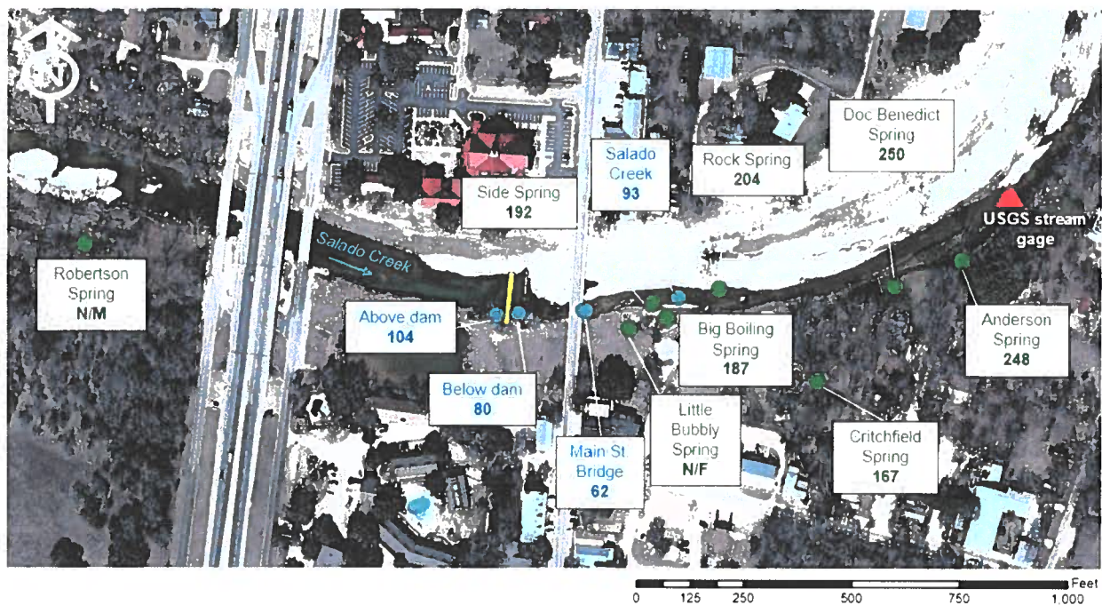
Figure 17: Synoptic radon-222 concentration in groundwater and surface water at Salado Springs. Radon-222 concentrations are given in pCi/L. The abbreviations “N/M” and “N/F” mean “not measured” and “no flow” respectively.
